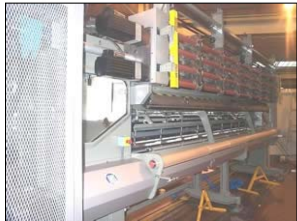
Cobble machines can be fitted with up to 2000 needles
